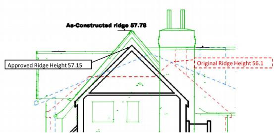
The large chimney, not shown on the original slice drawing is even taller. The original building height of 56.1 was not indicated on the previous application but can be
